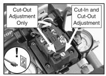
Figure 22. Pressure adjustment screws.
